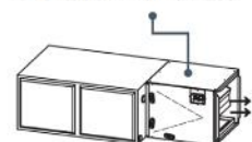
Horizontal cased coil orientation with furnace
